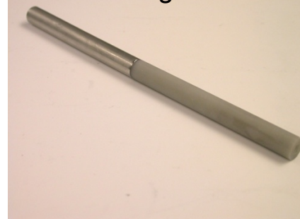
Figure 2: Modified MEMS-DCA package to support 800°C pressure sensor operation.
