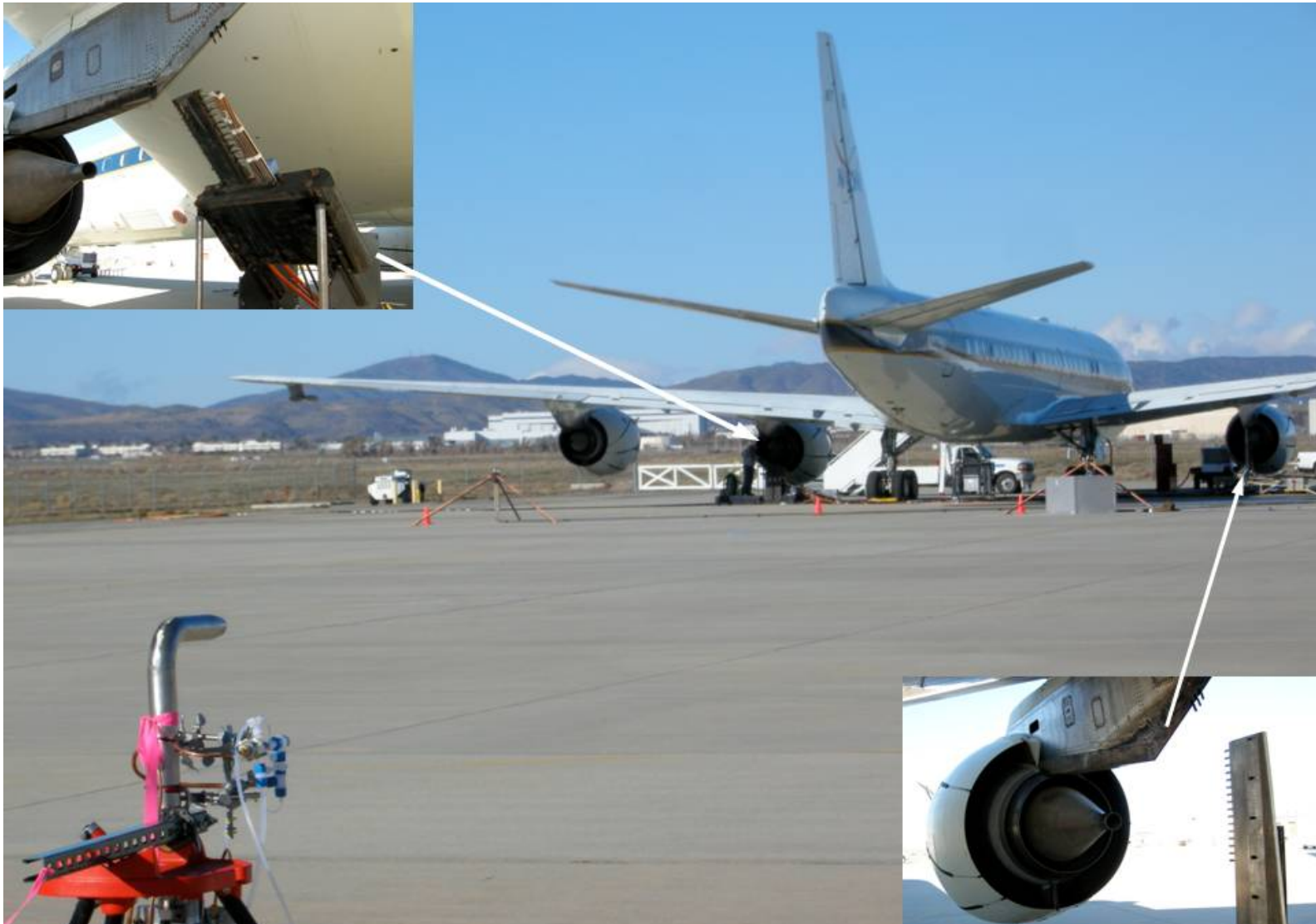
Identical 1 and 30 m inlets behind left and right inboard engines
