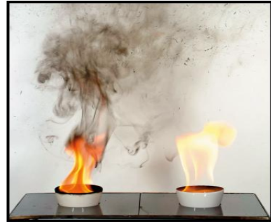
GTL's combustion (on the right) is less sooty
