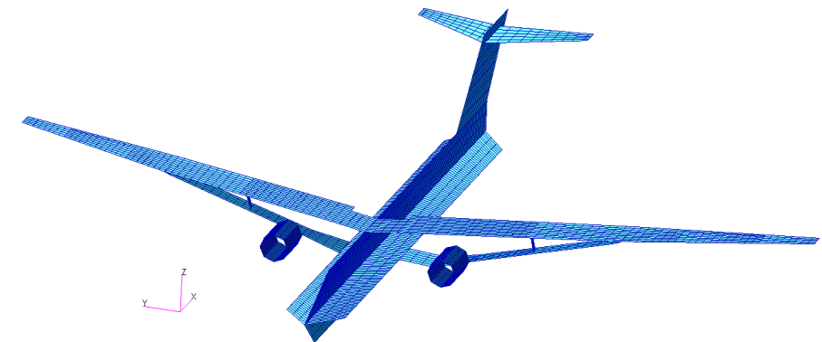
Doublet Lattice Aerodynamic Model with Refined Mesh
