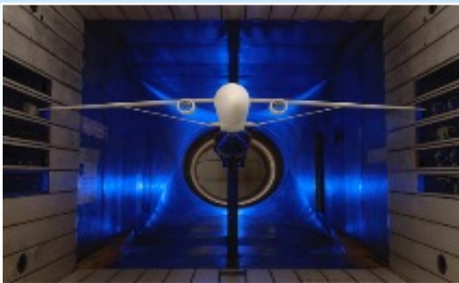
Transonic Truss-Braced Wing 5-10% fuel burn benefit
