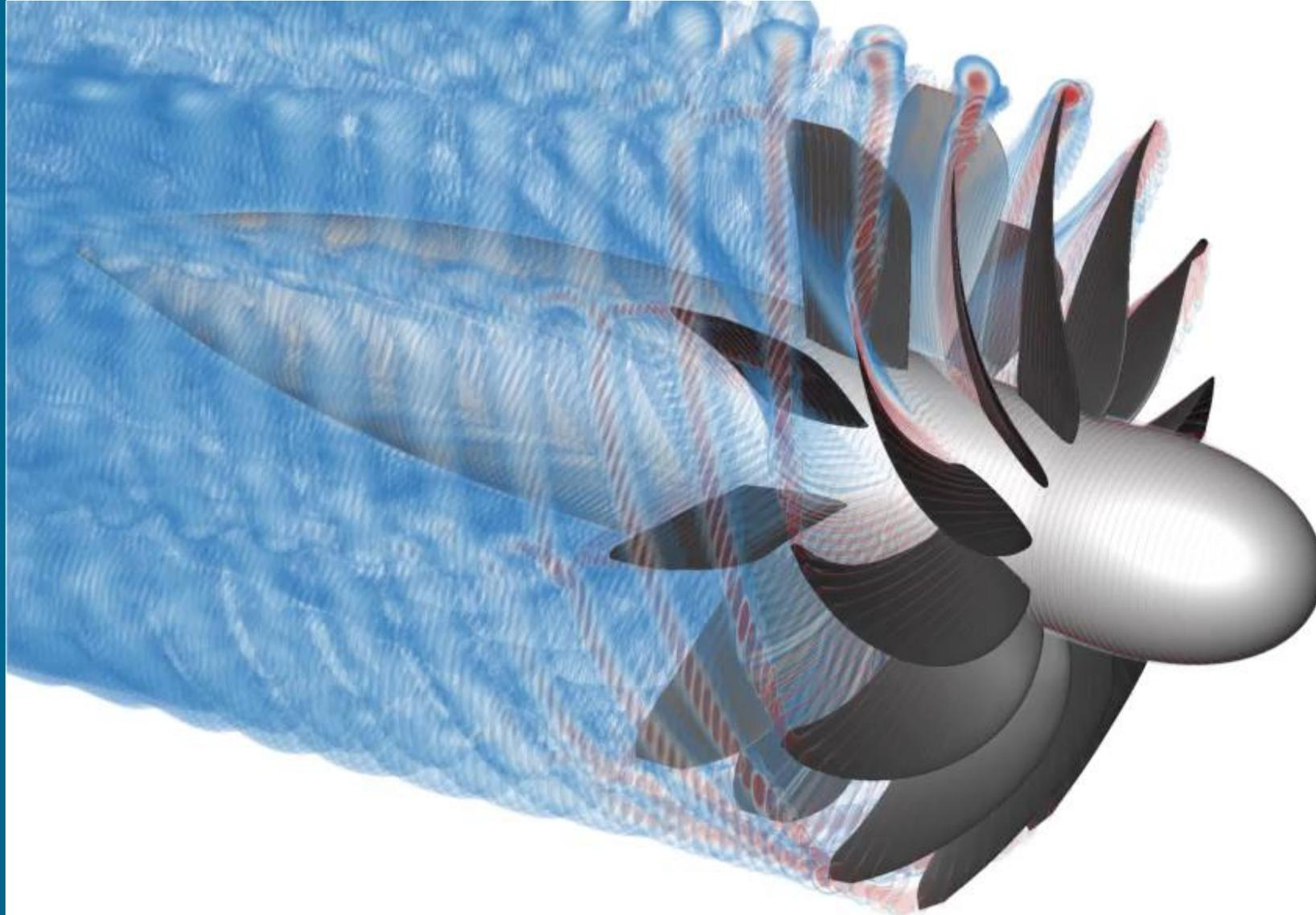
Open Rotor and Stator (ORAS) or Unducted Single Fan (USF) or Open Fan
