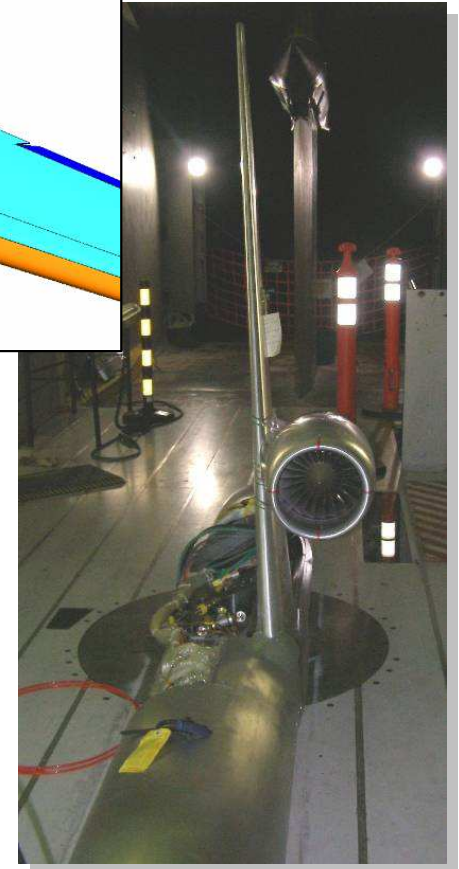
Wing/Nacelle Test Hardware in Ames 11'
