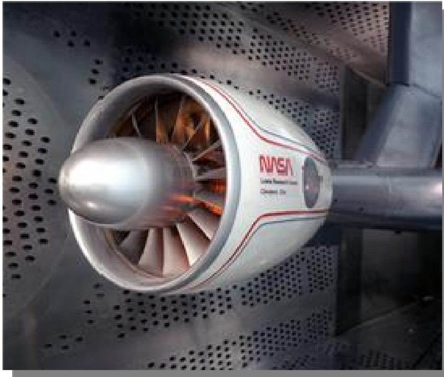
17" Advanced Ducted Propulsor in NASA Glenn 8'x6' Wind Tunnel
