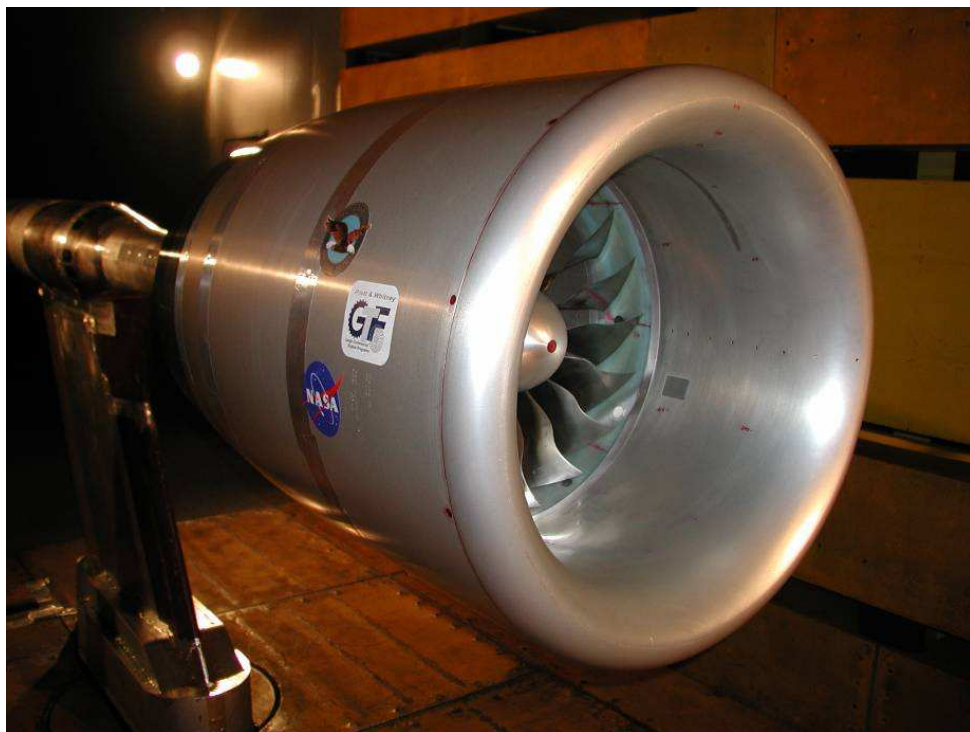
Pratt & Whitney Geared Turbofan Model in Glenn 9'x15' Wind Tunnel
