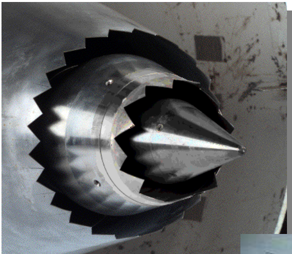
Advanced Chevron Test in NASA Glenn AeroAcoustic Propulsion Lab (AAPL)
