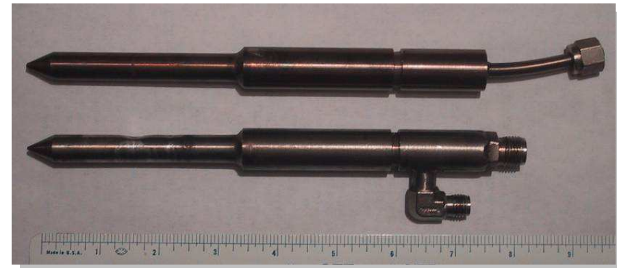
Exhaust Gas Sampling Probes
