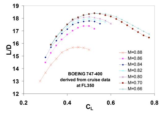
C<sub>L</sub> is obtained assuming that at cruise the aircraft is flying at L/D<sub>max</sub> and at conventional angle of attack
